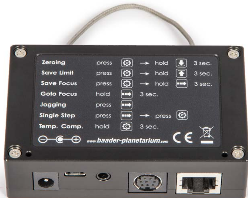
Overview of the functions of the SD II Controller – printed on the back of the controller.
