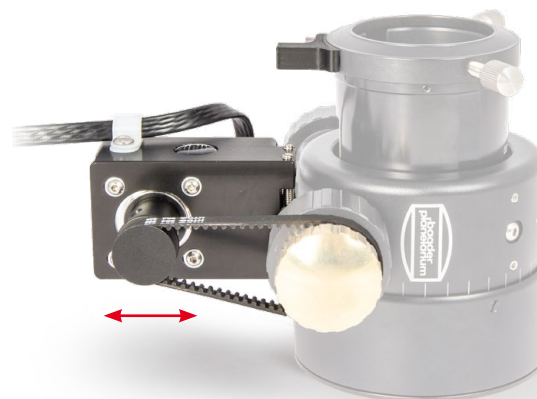
Img. 4: Move the motor inside of its housing until the toothed belt is under a good pressure.
