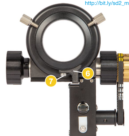
Img. 5: The magnet holder is attached instead of the lower clamping screw at the focuser tube. It must be parallel to the SD II.
